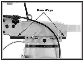
Figure 50. Exposing the ram ways for lubrication.
